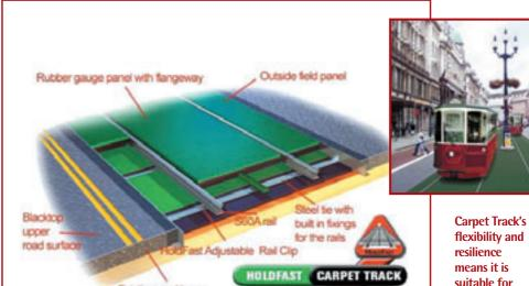
trams with up to a five-ton axle load.
